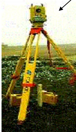
Station totale motorisée
